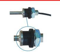
Temperature sensor with a mechanical fastening system without thread, with compression / expansion seal fixing. Mounting on wall of 2 to 6 mm thickness, through a hole of 22 mm diameter.
