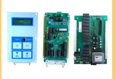
Microprocessor-based electronic unit for control and management of the process instrumentation in the Industrial field. Customized management programs.
