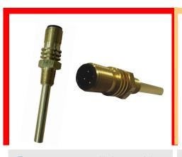
Temperature sensor with integrated heat sink to protect M12 electrical connection. Versions with measuring element Pt100, Pt1000, NTC, PTC..
