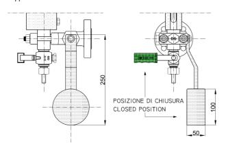
Code: LFC [Weight closing for lower handle] UFC [Weight closing for upper handle]
